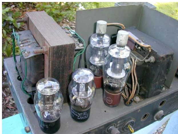
OT sandwiched between output valves and barriers.
